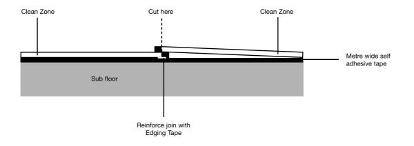
When joining Dycem you should always use Edging Tape under each join, as this will give a stronger bond. The two pieces of Dycem must overlap, cut through the two using a sharp knife and straight edge (as shown above) remove the cut pieces (shown in Black) to allow the Dycem to lie flat on the floor.
